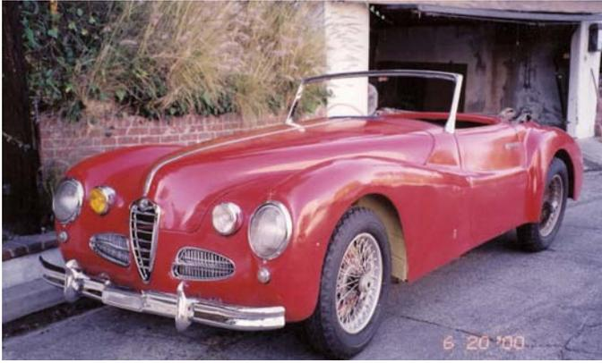
Alfa Romeo in California in 2000, with an Alfa 1900 grille, incorrect bumper and added extra headlights.
