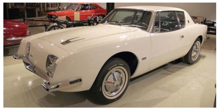
This 1964 Avanti has an R-3 Jet Thrust engine with a Paxton supercharger. It is certified to have been the last Avanti produced by Studebaker.
