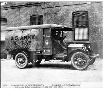
GMC built over 5000 ambulances on its Model 15 and Model 16 chassis. The one shown here was used for X-ray services, a new medical procedure in WWI.
