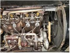
From the beginning Buick featured overhead valve (OHV) design for its engines, such as this D-4 motor used in ambulances sent to Europe.
