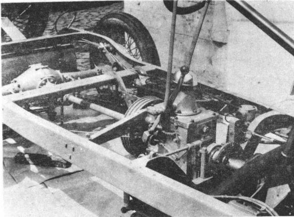
Behind engine - large drum behind transmission is the service brake. lever nearest camera is the emergency brake which worked on the rear wheels. The short lever between the gear-shift lever and the brake lever is a mystery. It seems to operate a dog-like mechanism in front of the transmission. This possibly may have been for the fourth gear.
