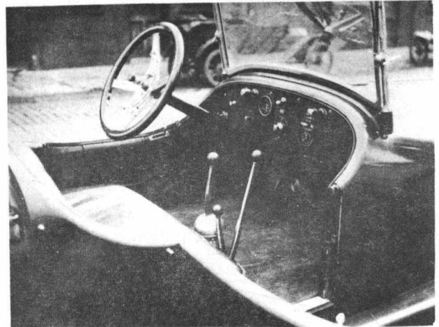
Interior of the ARGONNE showing simple and neat dash. Doors on this car have hidden hinges and this hints at above-average quality. The levers for the transmission and emergency brakes are shorter than shown on the bare chassis. Examination of all of these photos shows considerably more attention to detail than for most assembled cars of this period.
