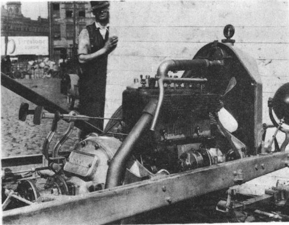
The 4-cylinder Buda engine with Argonne identification on valve plate and on clutch housing. Seen behind the clutch housing is one of the special universal joints mentioned in the technical description. Low on the side of the engine is the Eisemann magneto and the Westinghouse generator, connected in tandem. Fan was a casting. On manifold is the firing order, 1,3,4,2.
