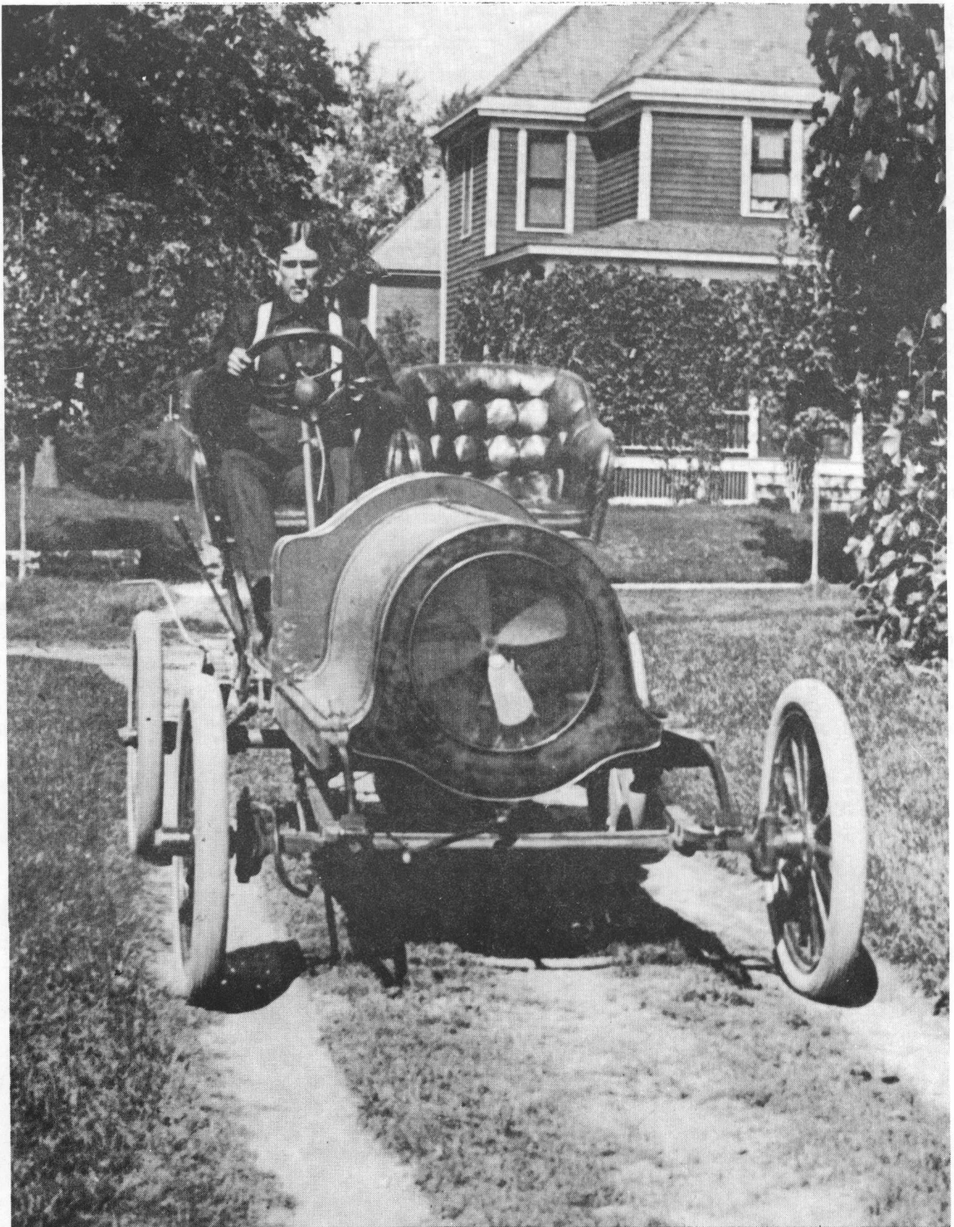
This is the four-cylinder air-cooled car built in 1904 and 1905. The motor had a 3\frac{3}{4} inch bore and a 4 inch stroke. The combustion chamber was designed so the incoming gas had to pass over the face of the exhaust valve which kept the valve cool and had much to do with the successful operation of this motor. The drive was thru a planetary transmission and bevel gear and final chain drive to the rear axle. Top speed of this car was about 35 miles per hour.
