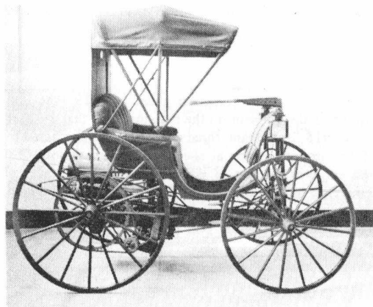
This is the first Duryea motor vehicle, designed by Charles E. Duryea in 1891 and 1892, and built by his brother, Frank Duryea, in 1892 and 1893. It was road-tested in September, 1893. Power to the rear wheels was supplied by a one-cylinder two-cycle engine through a friction transmission. Neither the engine nor the transmission performed to Frank Duryea’s satisfaction, and the car was rebuilt with a three speed and reverse spur gear transmission and a one-cylinder four-cycle water-cooled engine. This rebuilt car, shown here as it presently appears in the Smithsonian Collection of Automobiles and Motorcycles, was donated to the museum in 1920 and restored in 1958.
