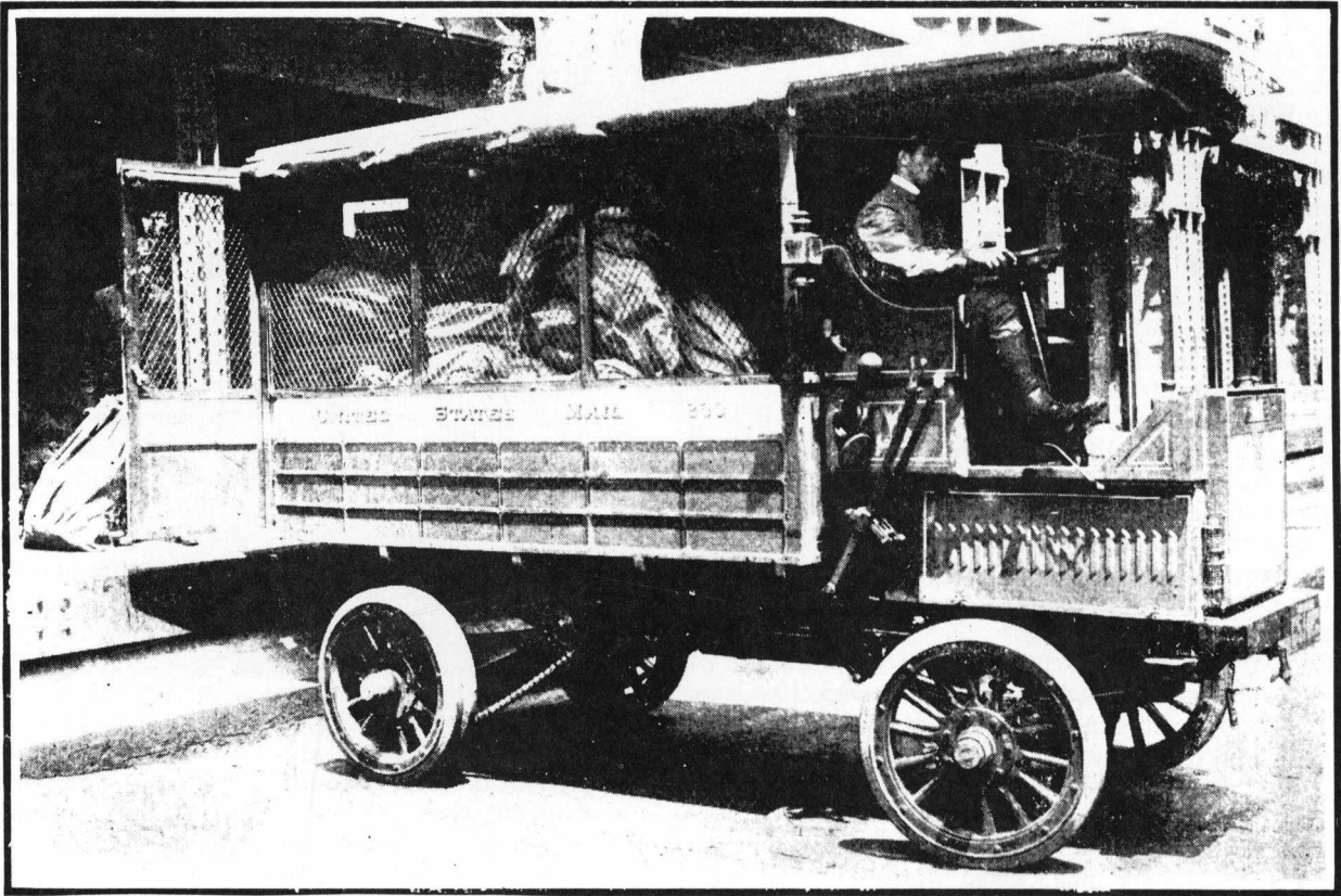
ALCO MODEL 2-T TWO-TON-TRUCK. This vehicle, manufactured by the American Locomotive Company, of Providence, Rhode Island, was one of a fleet of 80 ordered in the first half of 1913 for the New York City Post Office. Its 10-foot bed provided 34 square feet of loading space, propelled by a 32 horsepower four-cylinder engine at a speed of about 17 mph. The chassis, which weighed 4,500 pounds, was carried on solid tires, 36 x 4 inch in front, 36 x 3.5 inch dual at the rear. 1913 was the final year of production of this truck, for in September of that year the American Locomotive Company withdrew from the manufacture of automobiles and trucks, with a promise that parts and service for existing vehicles would be available for at least five years.
