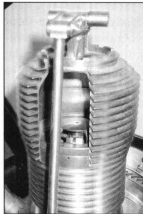
The seven-cylinder Gnome was the first reliable rotary aero engine. Its inlet valve was placed in the crown of the piston, as seen on the right, with compression holding it firmly closed on the firing stroke.
