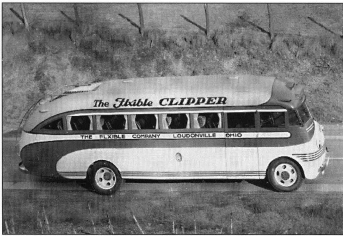
Fig. 9 - This 1937 Clipper represents the first year of Clipper production. The 1937s were also the first Flxible buses of the cab-over-engine design and the last to use wooden framework.
