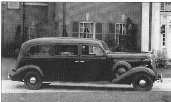
Fig. 8 - The 1936 Flxible-Buicks featured on an all steel "Turret Top" along with modernistic flowing lines.
