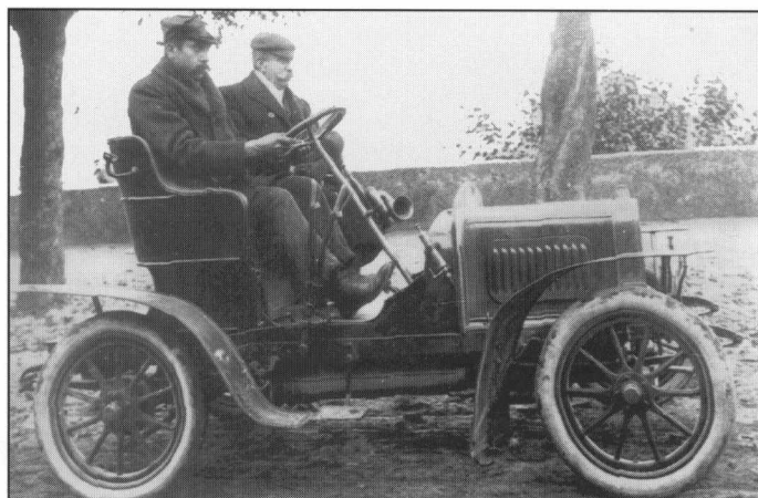
Fig. 4 – Laurin & Klement begins to build cars: its 1905 Type A with a 2-cylinder engine of 6-7 horsepower. (From Margolius & Meisl, Škoda Laurin & Klement )
