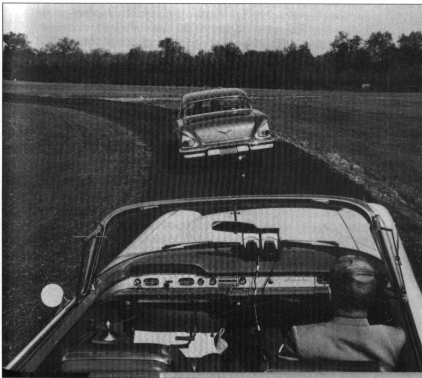
Fig. 3 – GM/RCA demonstration of a convertible Chevrolet Impala navigating a road course without driver or steering wheel.
