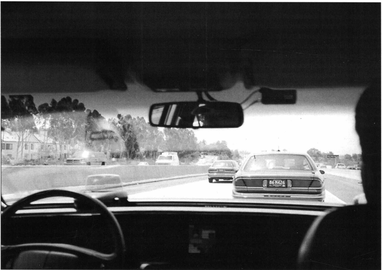
Fig. 6 – Photo taken from the backseat of a California PATH designed automated vehicle while taking part in a platooning exercise at Demo '97 in San Diego.
