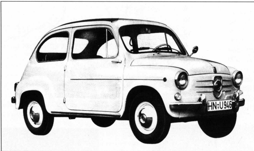
Fig. 7 – NSU Jagst 770. Note relocation of parking lamps.
