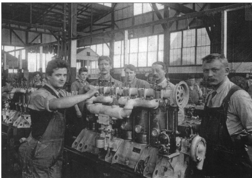
Fig 4 – Hall-Scott workers assemble an A-5, one of Hall-Scott's trailblazing aviation engines. The A-5 displaced 824.7 cu. in., weighed 525 lbs., and developed 125 h.p. @ 1250 r.p.m., rendering a power-to-weight ratio of just 4.2 lbs. per h.p. In the early 20th century, Hall-Scott was a recognized leader in American air power. (Francis Bradford Collection)
