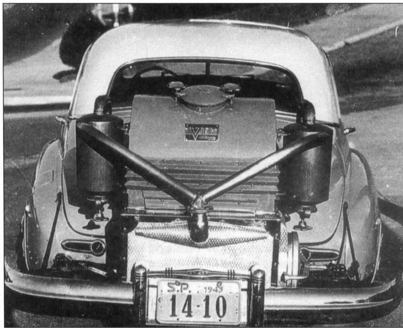
Fig. 5 – 1942 Buick equipped with GM gasogene conversion. (Courtesy ANFAVEA)
