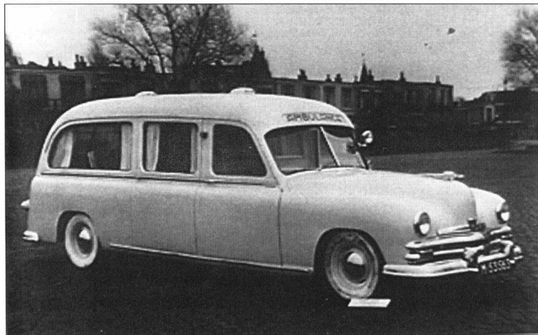
Fig. 5 – The ambulance constructed by Gebr. Visser on a 1949 Kaiser chassis.
