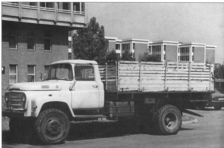
Fig. 2 – A stake-bodied Carpaţi truck, one of a variety of configurations, including dump bodies and trash haulers. The cab and V-8 engine resemble Ford's 1956 F Series, and for good reason since the design and production rights came from Ford.
