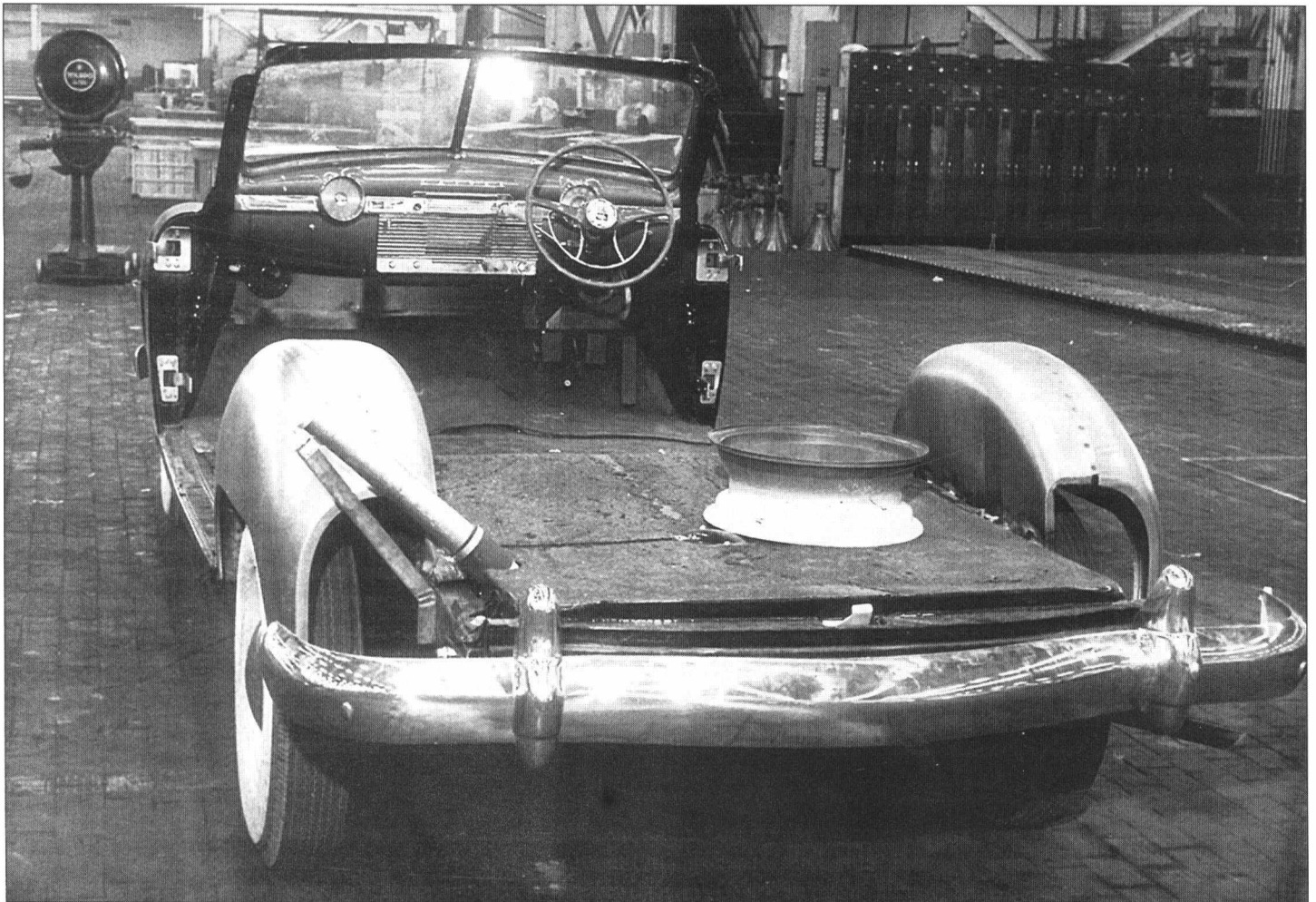
Fig. 7 – Incomplete 1949-50 Kaiser converted to right-hand drive.
