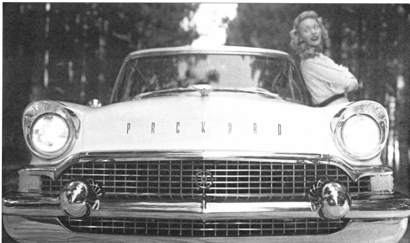
Fig. 2 – The 1957 Packard Clipper, the first to be manufactured in South Bend. It incorporated a Studebaker body shell and many Studebaker parts (from the editor's collection).
