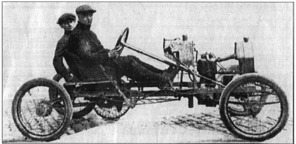
Fig. 5 – One of the two Violet-Bogeyes entered in the 1913 Cyclecar Grand Prix, their engines using aluminium-alloy pistons (supplied by the author).
