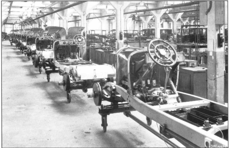
Above, construction of chassis using assembly dollies at Untertürkheim, 1925. Below, certificate of the Daimler-Benz merger, 1926. Daimler AG
