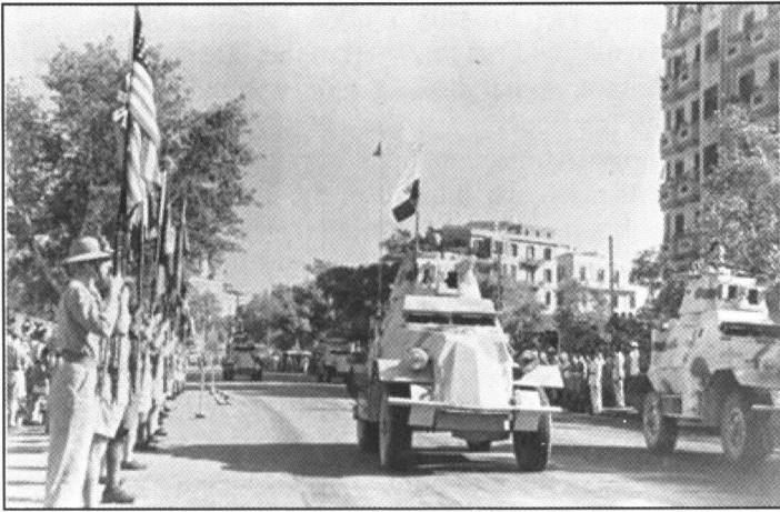
Ford-based Marmon-Herrington armored cars developed in South Africa were widely used in World War II.
