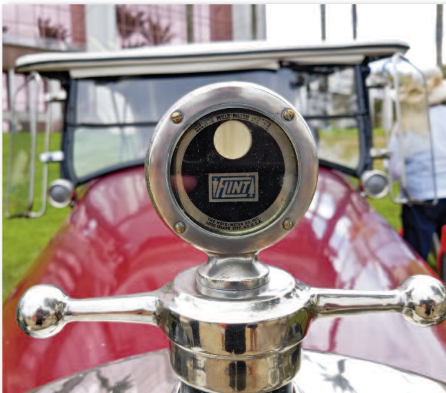
Figure 13: A marque-specific Moto-Meter, as installed on a 1923 Flint Sport Touring. Photo by Don Keefe.
