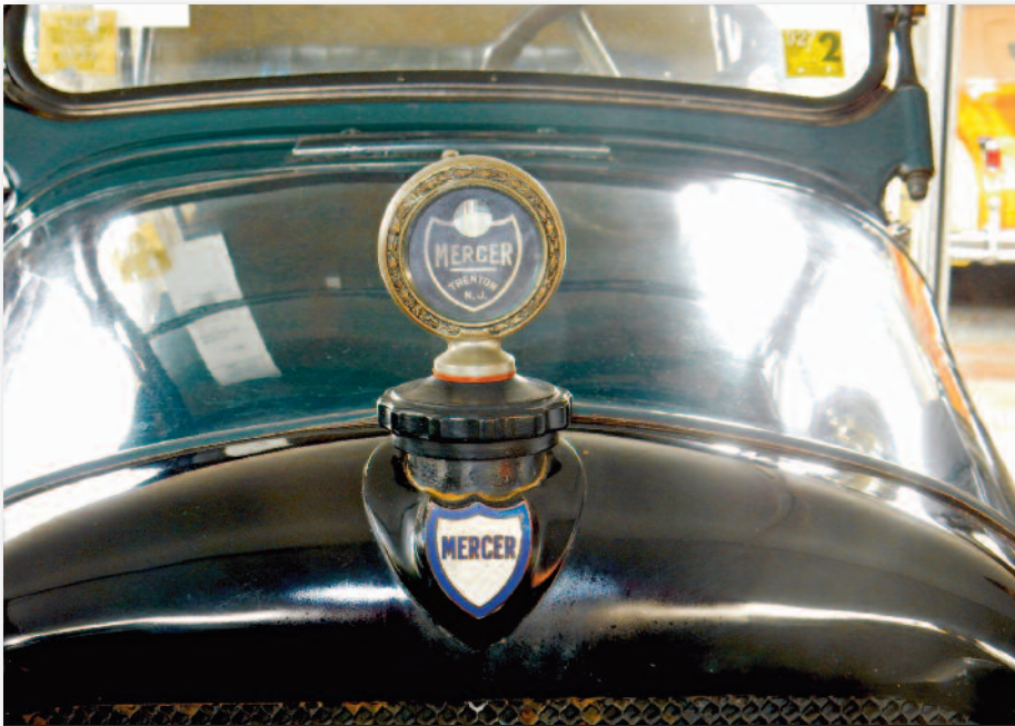
Figure 10: 1922 Mercer Series 5 Sporting with a Moto-Meter installed.
