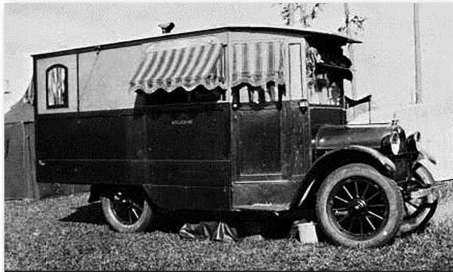
Figure 2: House cars were often home-built on automotive chassis and had varying levels of workmanship and finish quality. 17 Photo courtesy of www.floridamemory.com .
