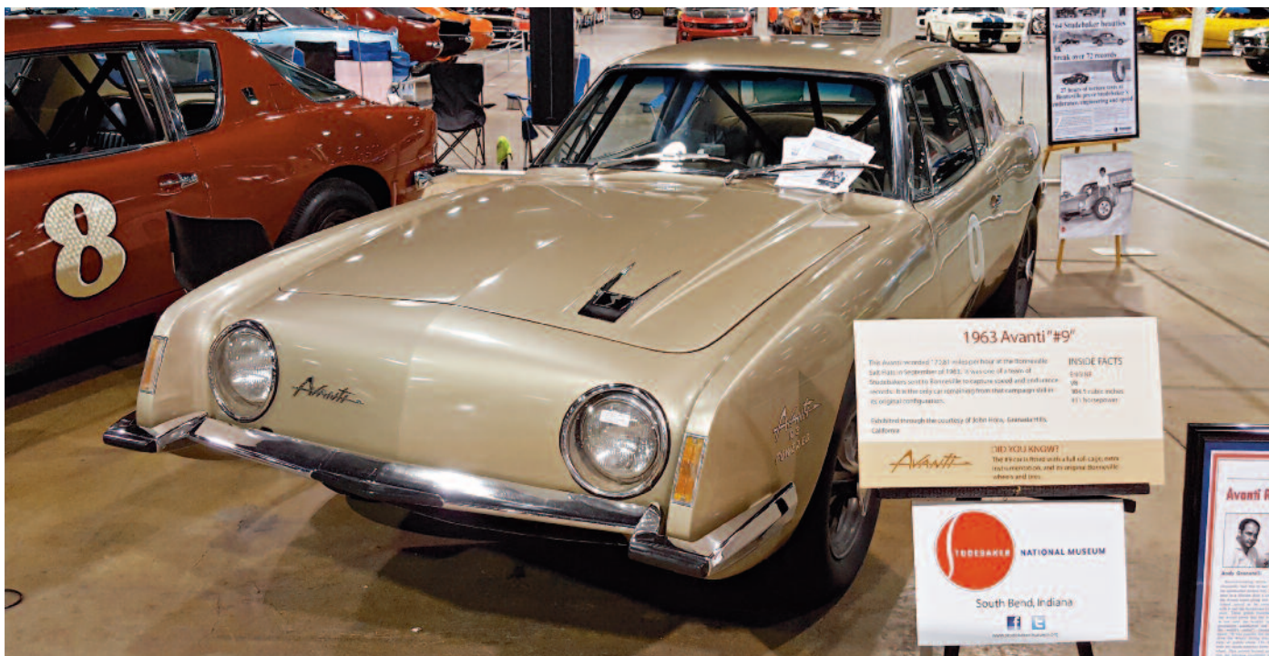
Fig. 7: One of the most exciting Studebakers ever built was this 1963 Avanti, known as #9. It featured a 304.5 cubic-inch, supercharged Studebaker V-8 rated at a whopping 411 horsepower. It was tested at Bonneville Salt Flats in Utah where it achieved a top speed of 170.81 mph. It was part of a factory-backed team and is the only one left still in its original race configuration. Photo by Don Keefe.
