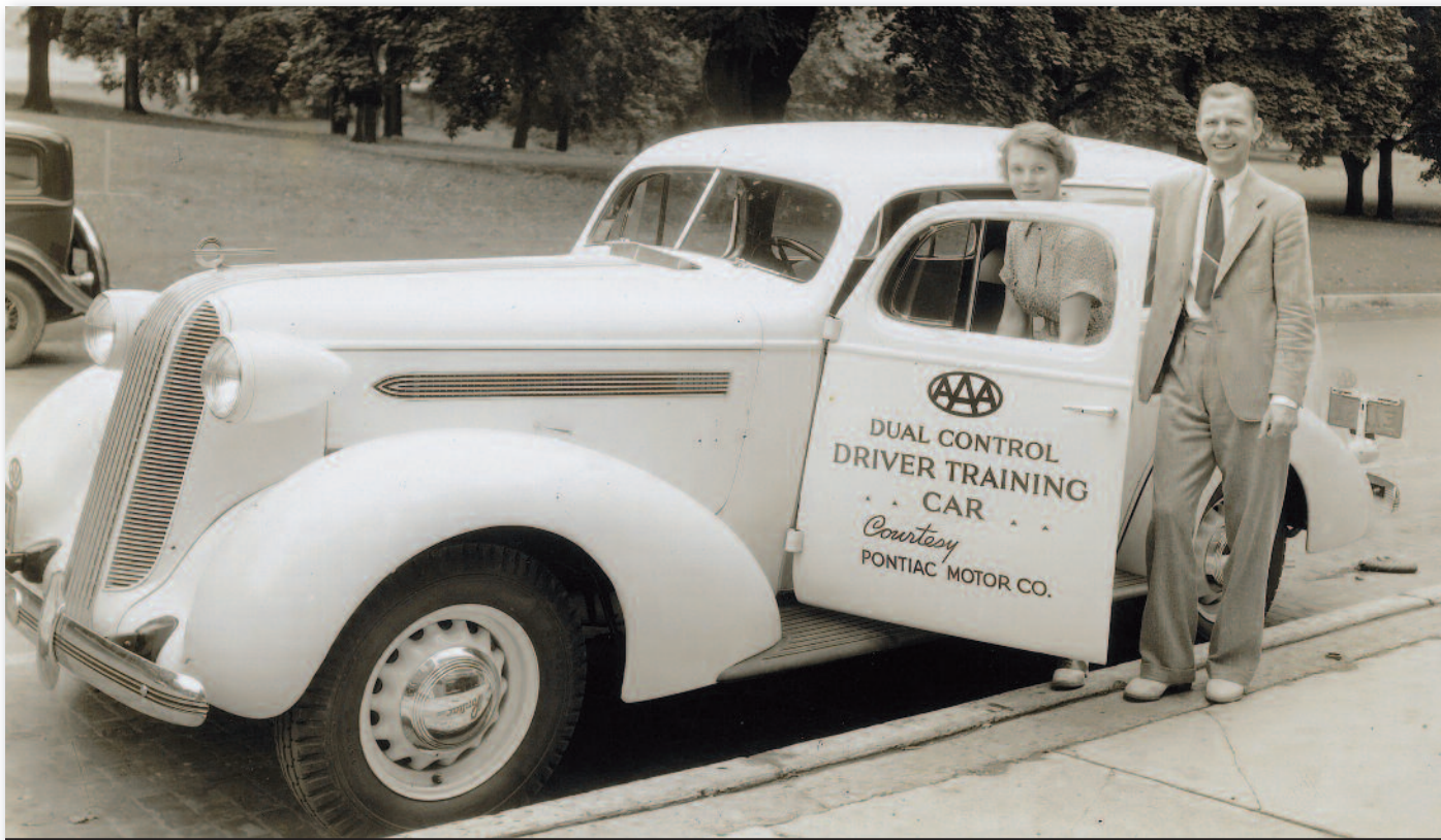
Amos Neyhart is seen here with a student and a 1936 Pontiac four-door sedan fitted with a dual-driver control system. Photo courtesy of Penn State University Archives.
