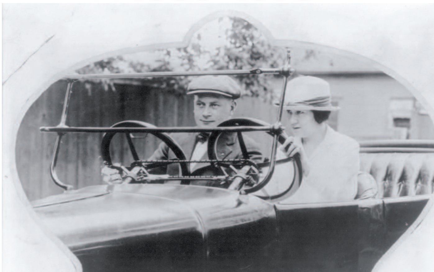
Student and instructor in Briscoe automobile—notice the dual controls. August 4. 1917. (Library of Congress).
