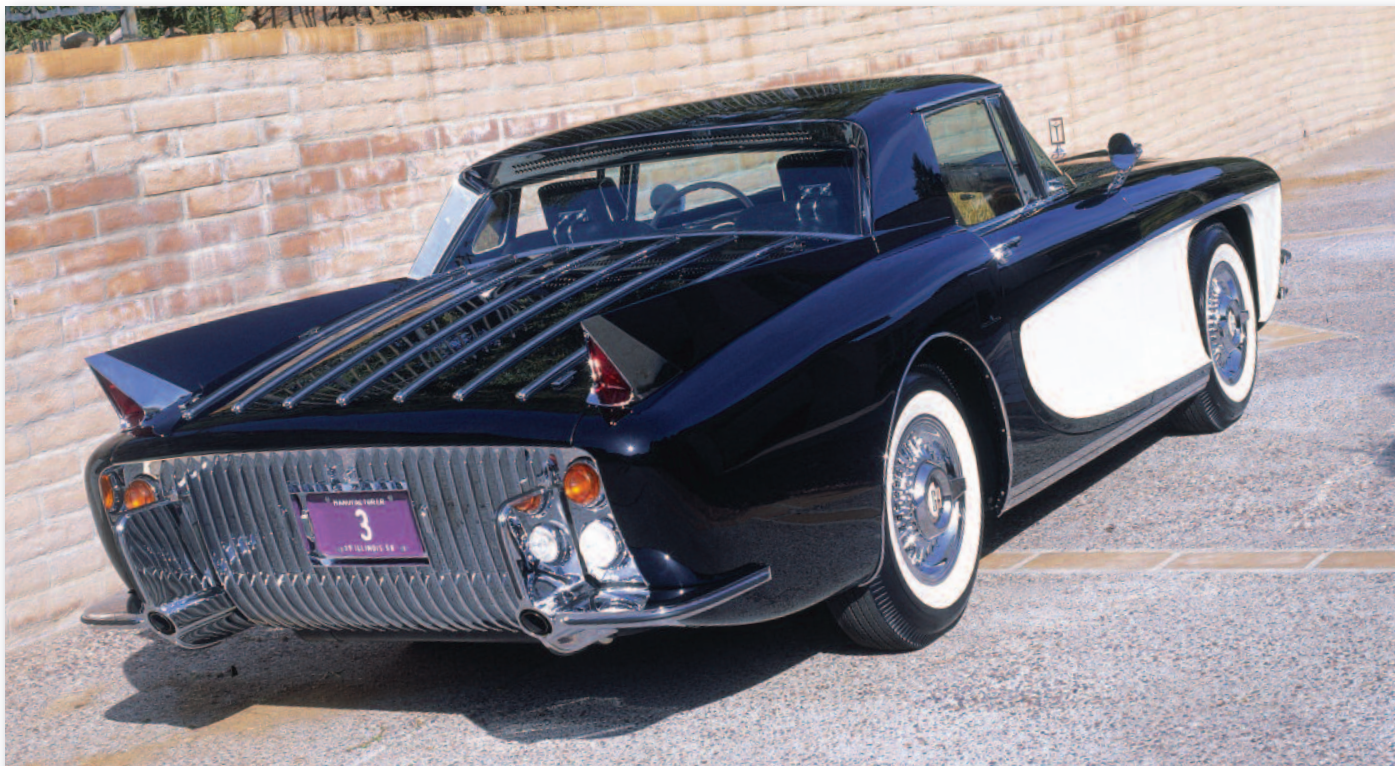
Figure 17: The ribbed, bottom-hinged rear panel hid a slide-out tray containing the spare tire.
