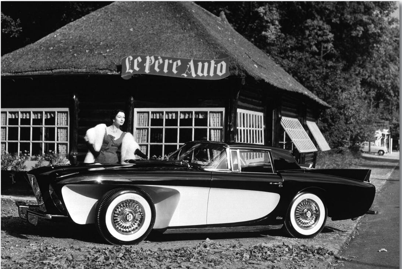
Figure 3. This side view of the original Spohn-bodied showcar shows the unusual contour of the front wheelwells. It was definitely a case of form at the expense of function. Windshield frame accepted 1955 Thunderbird glass.
