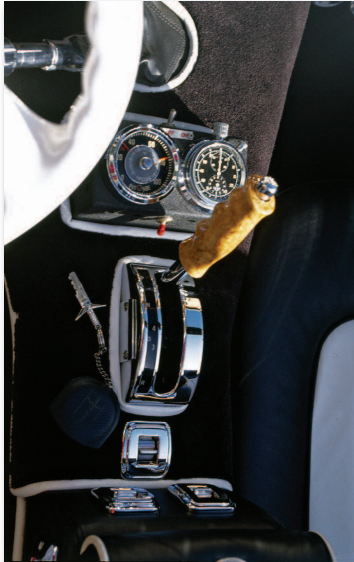
Figure 14: Hydra-Matic transmission is controlled by a floor shifter. A Heuer chronometer is mounted in the console ahead of the shifter.
