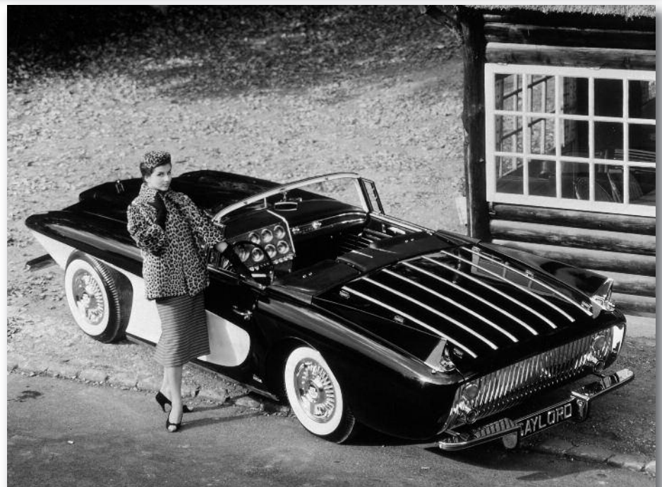
Figure 4: A retractable hardtop filled the trunk so a rack was mounted on the rear deck to carry luggage. Figure 5 (overleaf): The final Gaylord body design was more practical than the first prototypes, featuring quad headlights and fuller front fenders, as well as stouter front and rear bumpers.
