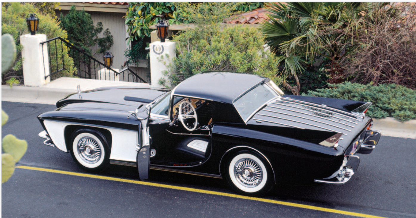
Figure 18: Even with a wheelbase of just 100 inches, the Gaylord was designed to be a roomy two-seater. It shared its “Sabre-Spoke” wheels with the 1955 Cadillac Eldorado, but added unique center caps.
