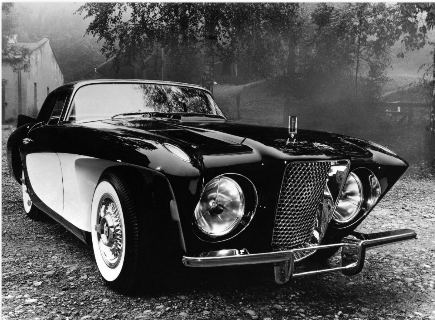
Figure 2: The first two Gaylords had Gordon Kelly-designed bodies built by Karosseriefabrik Hermann Spohn of Germany. Unique to the Spohn cars were large Lucas P-100 headlights and scooped-out front wheel wells. The headlights would probably have violated American regulations, and the open wheel wells would have been difficult to keep clean.
