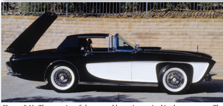
Figures 8-11: The operation of the retractable top is seen in this photo sequence. The retractable hardtop used an electric motor to lower the top under the rear-hinged decklid. The Gaylords compared notes with Ford engineers working on the Skyliner.
