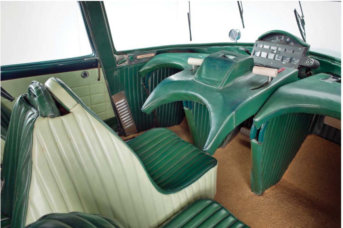
Figure 5: Center located driver's seat with left/right levers replaced the standard steering wheel. There was a large block of padding between the levers to cushion the head and chest areas. Driver and front passengers were located back from the windshield to minimize windshield glass contact in a crash. (Used with permission by the THF.)
