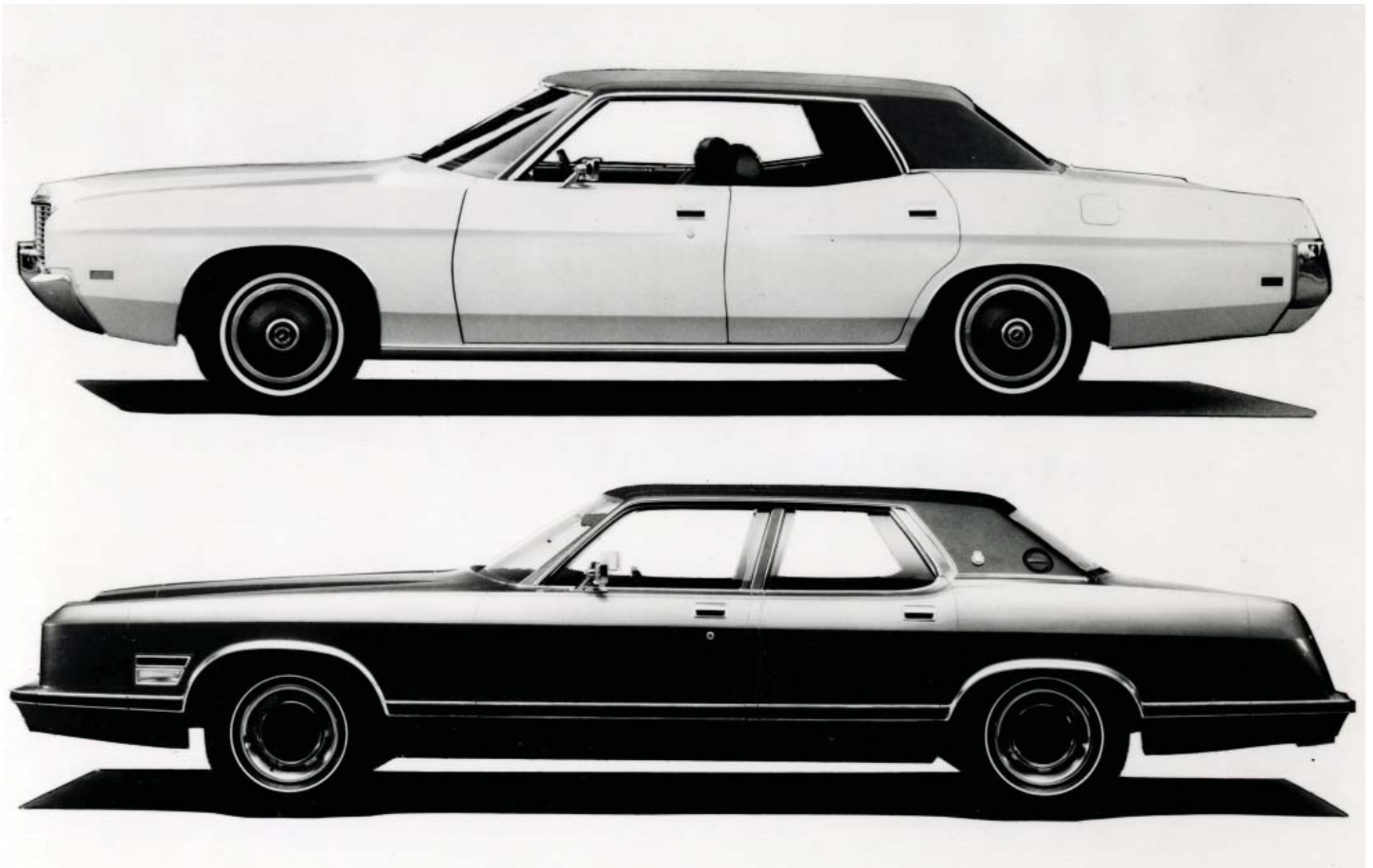
Figure 8: 1971 Ford Experimental Safety Vehicle, was a modified production 1968-1969 Ford Galaxy 500 and is shown in the lower figure compared to original production car in the upper figure. The extended front-end on the ESV reflects the extra crush distance needed to absorb the 50-mph barrier impact energy. The rear deck or trunk appears to be shortened and the whole greenhouse moved to the rear. Note the B-pillars were put back in place for roof crush resistance in rollovers. The front chassis/ frame members employed what were called “plastic hinges” to help absorb a majority (65%) of the frontal crash energy and the body sheet metal absorbed (35%) of the energy. Overall, the objective of designers was to keep the ESV’s stylish, attractive and aesthetically pleasing. 51 (Used with permission by the National Automotive History Collection, Detroit Michigan.)
