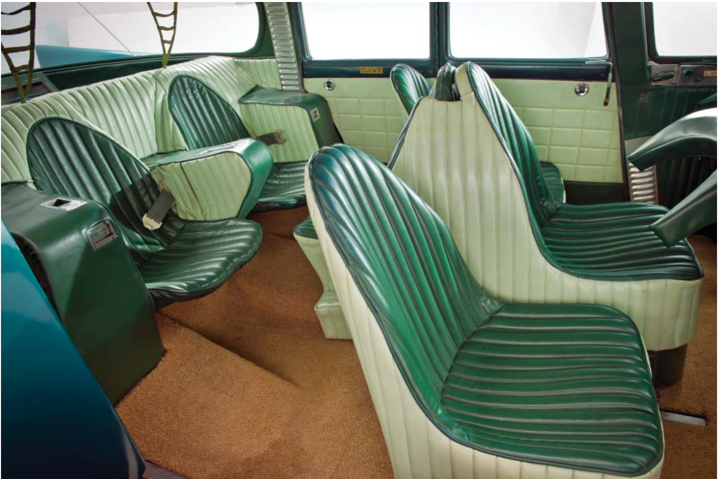
Figure 6: Rear seat compartment with center, rearward-facing passenger for a child to reduce passenger head contacts in a crash. Note the built-in seat belts and anti-whip lash nets for the forward-facing back seat passengers. (Used with permission by the THF)
