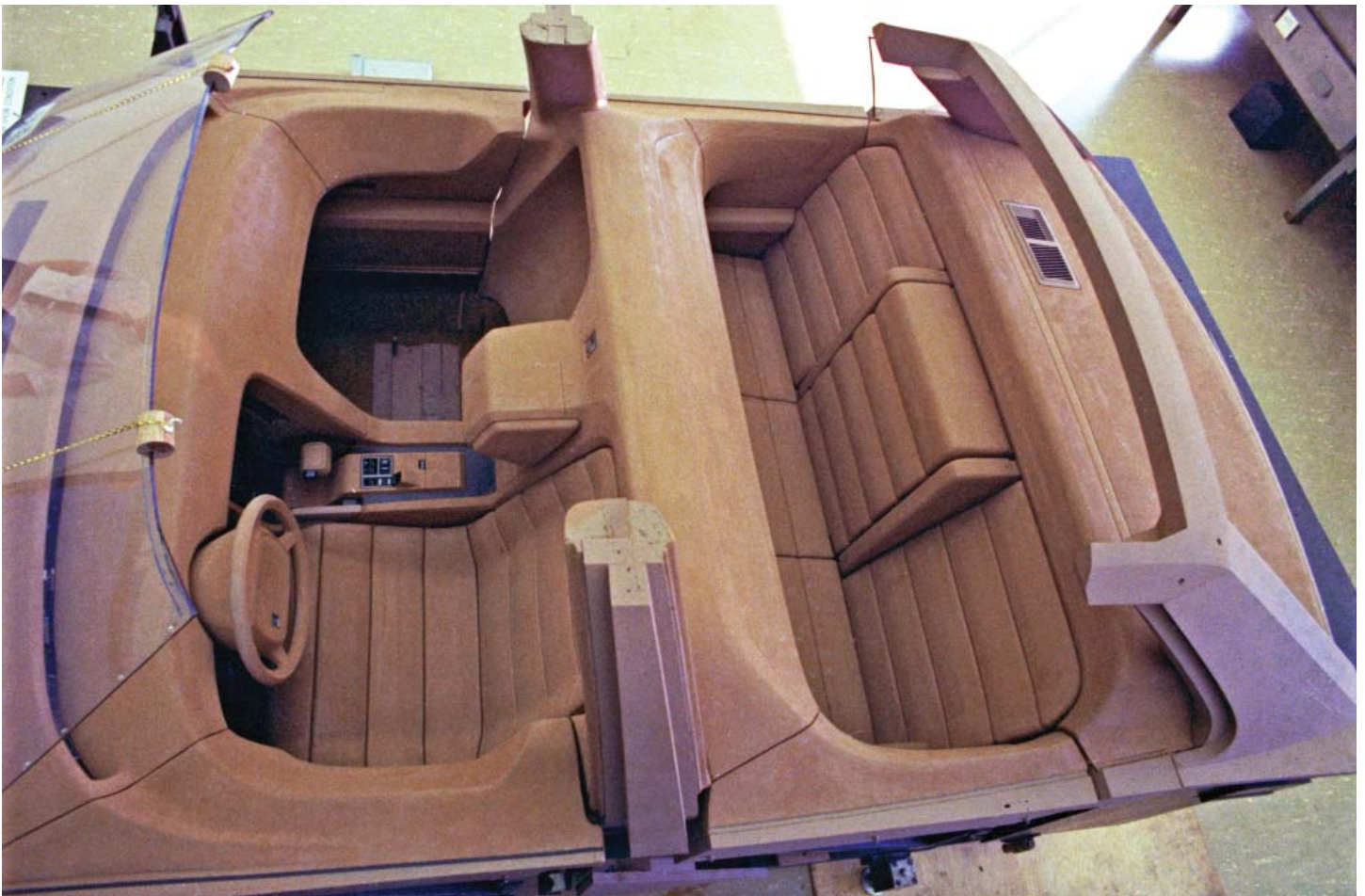
Figure 10: This is believed to be mock-up of the 1971 GM ESV (with roof removed) to show the interior padding anticipated for passengers to survive a 30-mph crash without their seat belts and a 50-mph crash with air bags. There is a padded bolster or padded partition between the front and rear occupants which contains the rear occupant air bags. The padded bolster also prevents the 30-mph unbelted rear occupants from flying up and over into the front seating area. (Used with permission by GMMA, Detroit MI)
