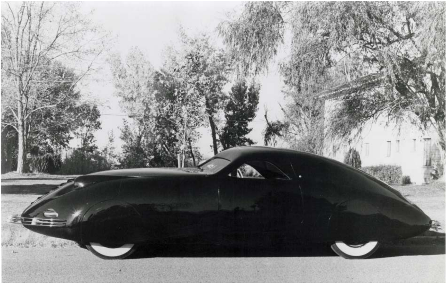
Figure 1: The 1938 Phantom Corsair designed and built by Rust Heinz and Maurice Schwartz, was a 4-passenger aerodynamic prototype built on a 1937 Cord-L chassis and distinguished by its unusual engineered provisions for high speed (122 mph), safety and comfort. The interior was lined with rubber slabs, seats were molded rubber without springs and interior walls were lined with ¾ inch cork composition. There were layers of sponge rubber under the upholstery. The steel “crash” board was covered with 2-inches of rubber covering so the occupants were sound and shock-proofed. The bullet-proof, tinted windows were slanted to eliminate driver glare. Many of these intuitive safety ideas were proven to be effective and became state-of-the-art knowledge by the mid-1950s and later. (Used with permission by the National Automotive History Collection (NAHC), Detroit Free Library, Detroit MI)
