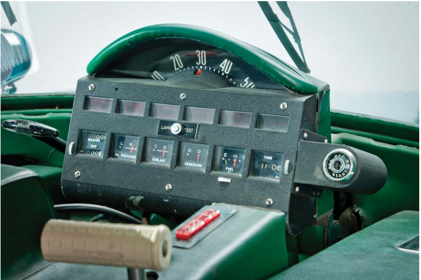
Figure 7: The instrument panel was located above the cowl line, just below the driver's line of sight, to minimize "eyes-off-the-road" time.
