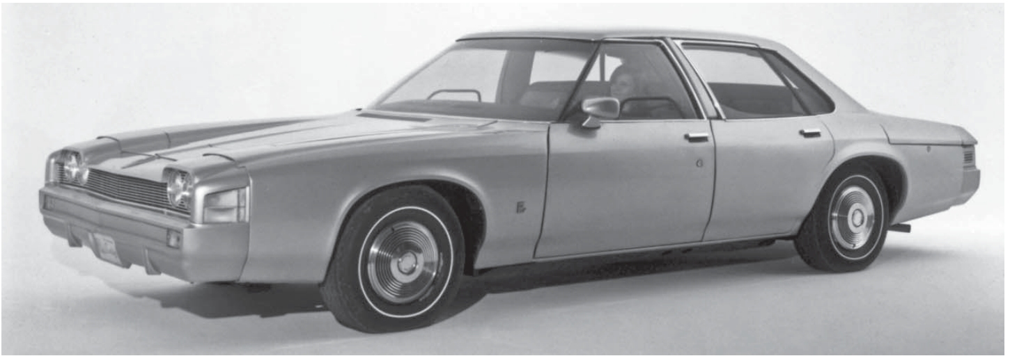
Figure 9: 1971 GM ESV. To off-set the weight of a heavier frame structure, the body of the 1971 GM ESV was made of aluminum. The front fixed windows had ports for added air circulation and access to external parking or toll road ticket equipment. The front-end nose and rear end were designed to absorb energy at low impact speeds (up to 10 mph) with a zero-body damage tolerance and subsequent minimal harm to pedestrians. 52 (Used with permission by GMMA, Detroit MI.)
