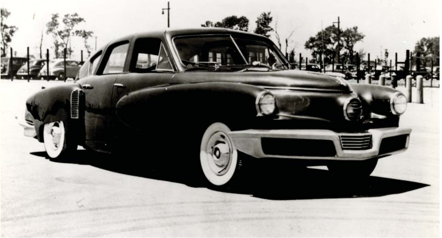
Figure 2: According to the Chief Designer, Alex Tremulis, adoption of the Tucker features alone might have saved 10,000 lives a year and there might never have been a need for US DOT/NHTSA. He called this car “Tucker, Symbol of Safety.” It was a six-passenger car with 4-wheel independent suspension, aircraft-type disc brakes for panic stops, rigid box frame with massive bumpers, sealed water-cooling system and 335 c.i.d., aluminum rear engine. Also, acceleration of 0-60 mph in 10 seconds, 0.28 drag coefficient, 122 mph top speed, 17 mpg and a price tag of $2,245. The design included a padded dash and recessed knobs and levers, but seat belts were not included. The Tucker sales department was opposed to the latter. The car had a centrally located headlight synchronized with the steering-wheel movement yielding a broader nighttime field of view. A curved, laminated pop-out windshield was in the offing for later models of the car. Many of these features were unheard of in any post-war American cars. These ideas have gained traction today among safety researchers. (Used with permission by the NAHC, Detroit Public Library, Detroit MI)
