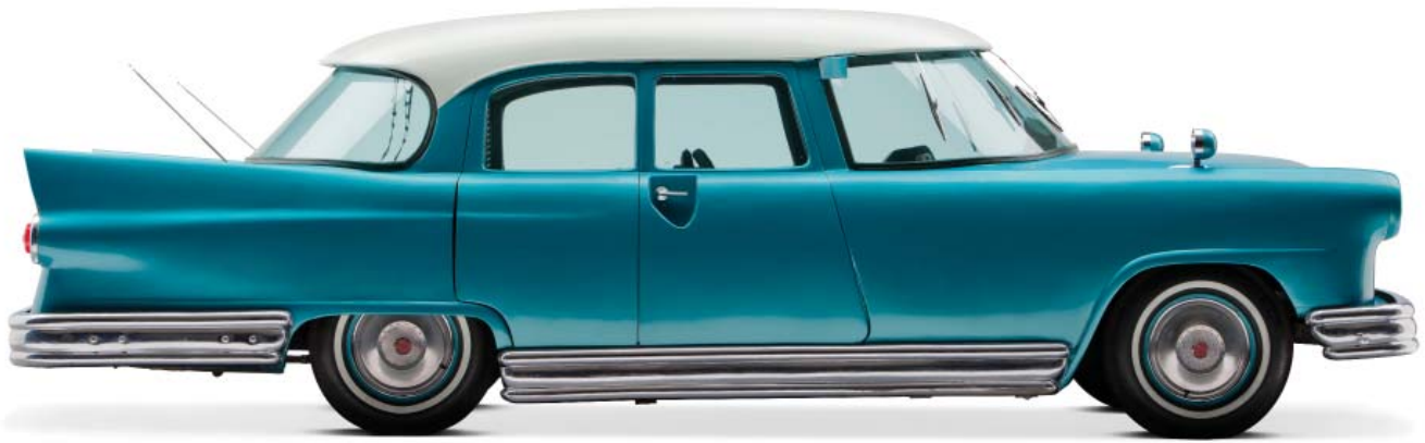
Figure 4: 1957 Cornell-Liberty Safety Car designed by Raymond Loewy, built by Ford Motor Company and sponsored by Liberty Mutual Insurance Company. This was a prototype car designed to show-off the latest safety technologies and was used as part of a U.S. auto safety promotion campaign. The A-pillars have been reconfigured to maximize driver visibility and the roof is cantilevered from there forward. The driver and front passengers are seated longitudinally aligned with the A- pillars. The door folds to provide access to both front and rear passengers. The high domed roof was designed for headroom, but accommodated the rollover structure for front and rear passengers. Outside rearview mirrors were visible to the driver via a large distortion-free windshield. The driver and front passengers were located a considerable distance from the instrument panel and windshield glass. (Used with permission by THF)
