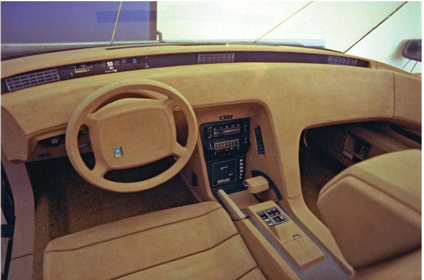
Figure 11: Interior front seat mock-up of the 1971 GM ESV showing the front occupant padded crash protection areas. A high mounted bolster separated the driver from the front seat passenger (See image right-hand, lower corner). Driver controls were recessed and hard knobs, buttons or protrusions removed so the interior surfaces were flush and smooth. The steering wheel had a large central padded area to distribute driver chest loads in the 30-mph unbelted crash test scenario. Air bags are hidden within the steering wheel hub for the driver and the right-hand dashboard area for the passenger for the 50-mph crash scenario. Also, note driver head-up display at the bottom edge of the windshield. (Used with permission from GMMA, Detroit MI.)
