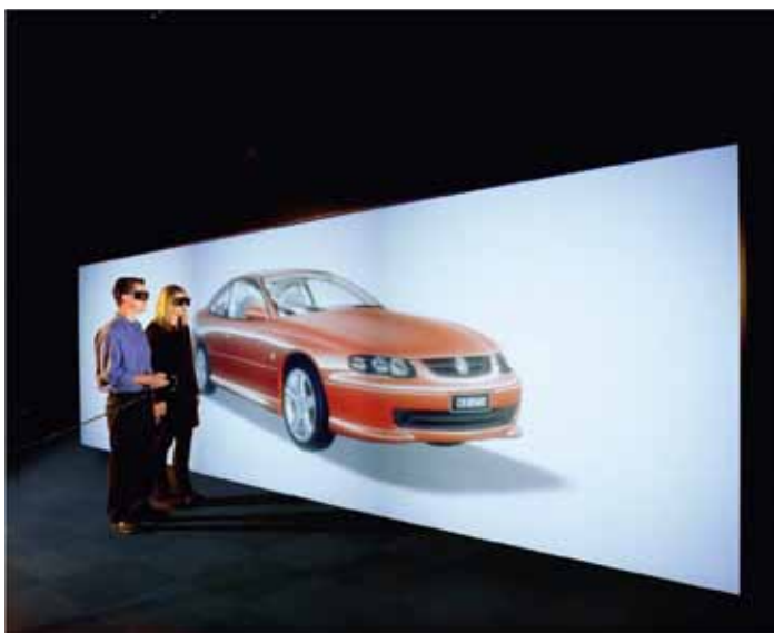
Holden VR Studio. Each design center had a VR studio having realistic full size virtual models viewable from any angle, with 3D glass if desired.
