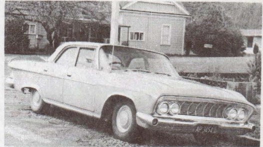
It looks like a Dodge but it's a 1961 export DeSoto produced by Chrysler Canada.
