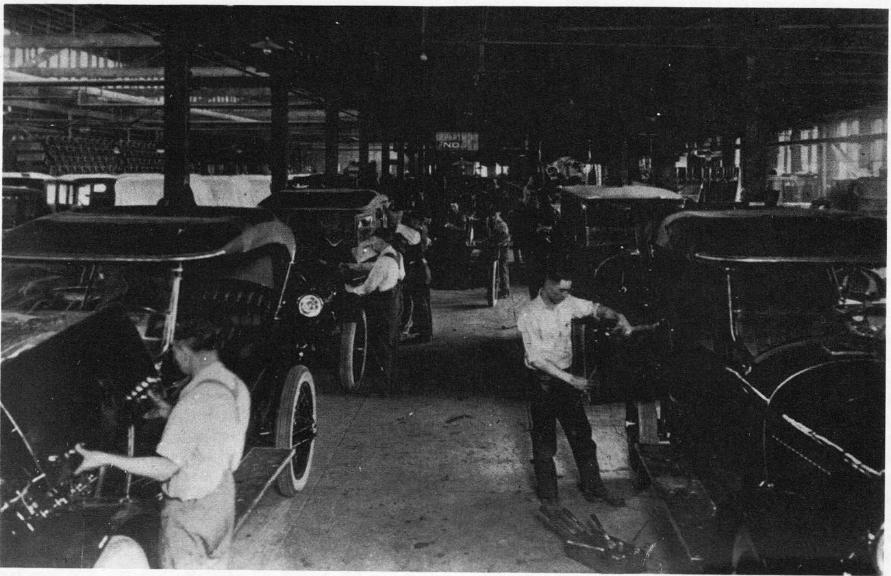
Scene in the factory of the Apperson Brothers Automobile Company, Kokomo, Indiana, about 1923. Apparently the cars were pushed along on their own wheels, without benefit of a moving assembly line. Note that the two cars in the foreground do not yet have their rear fenders attached. Photo courtesy of W. S. Huffman, Kokomo, Indiana.
