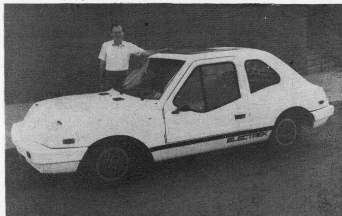
This front-wheel-drive ELECTREK has a top speed of 75 mph, and a city driving range of 75 miles at moderate speeds.
