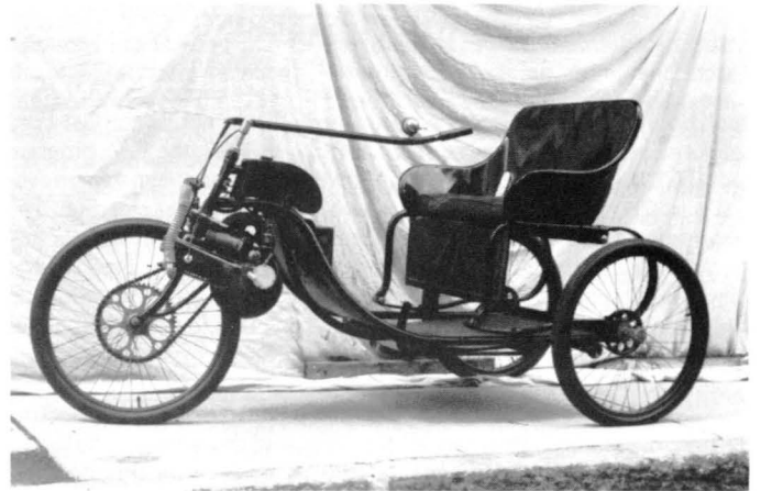
Richard Friedman's restored 1902/4 Dickinson Morette. Note that the rear axle is firmly fixed to the tubular frame, while the seat is suspended on leaf springs.
