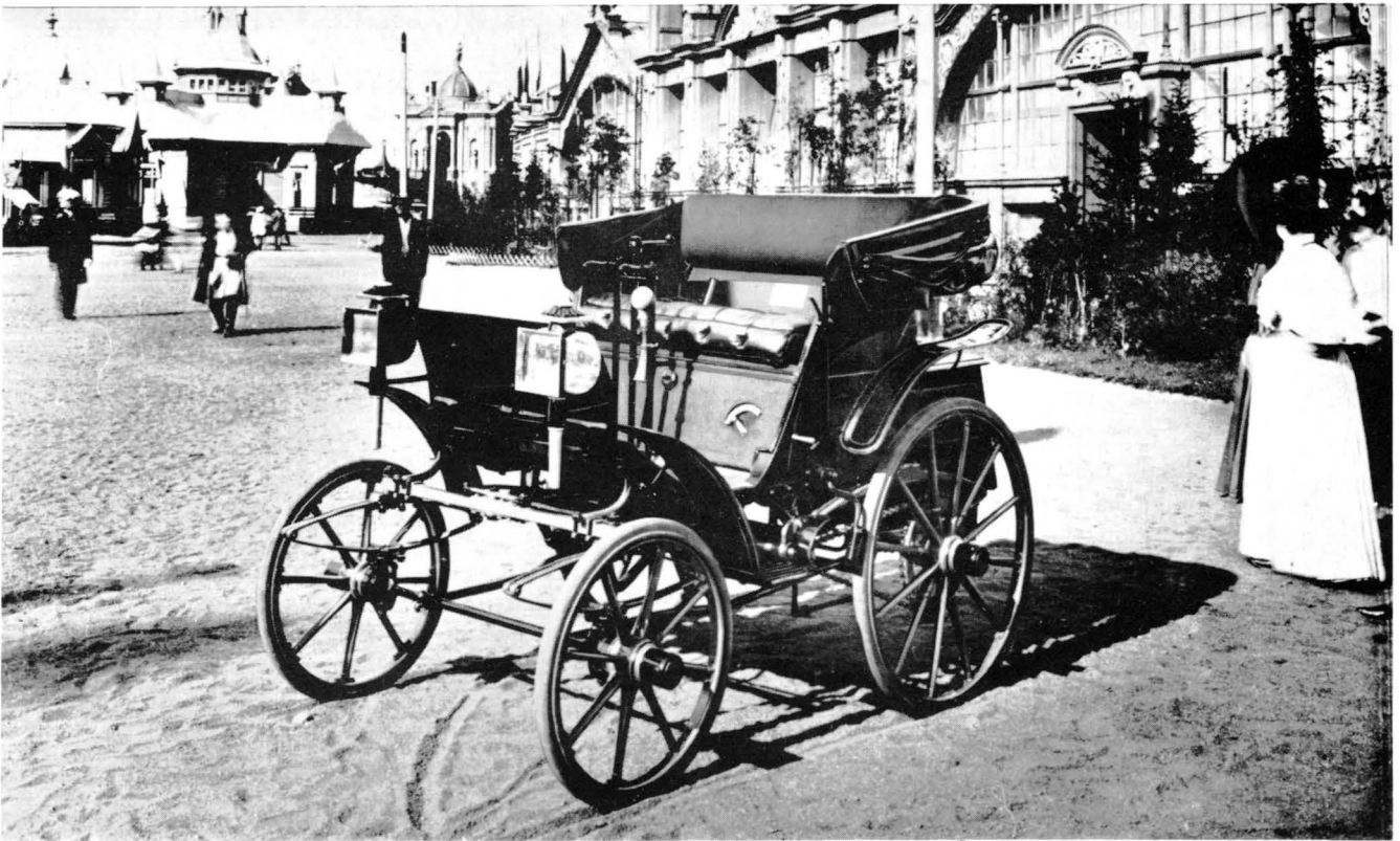
"THE PIONEER OF ALL RUSSIAN AUTOMOBILES" is the way Bill Emery describes the Yakovlev-Freze in Georgano's New Encyclopedia of Motorcars 1885 to the Present. Built in 1896 at the E.A. Yakovlev Works in St. Petersburg, the car is propelled by a single cylinder 2 hp engine located at the rear and driving through rubber belts. It was displayed that year at the Industrial Exhibition at Nijny-Novgorod. Photo courtesy of Soviet Life via Marshall Naul.
