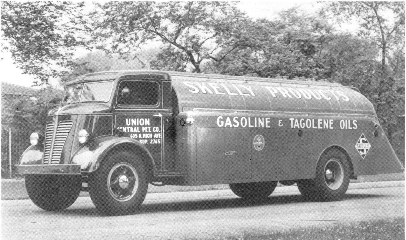
FEDERAL CASE: The 1930s produced some stylish trucks, of which niche manufacturer Federal Motor Truck Company had its share. This Federal Model 8911 carries a 2030-gallon, seven compartment tank by the Butler Manufacturing Company of Kansas City. Cab-over-engine trucks were introduced to the Federal line in 1937, so this photo must date from that era. Walter Gosden collection.
