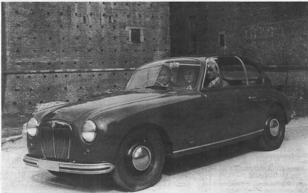
OHSAYCANYOUSEE? Very well, indeed, thanks to the voluptuous windows in our Panoramica. The body is, of course, by Zagato, its recessed door handles and flush window surrounds presaging modern practices. The Panoramica design was applied to several makes of chassis, this one being hinted by the grille. Did an MG TC ever look so aerodynamic, and what about that three-abreast seating? Peter Marshall collection.
