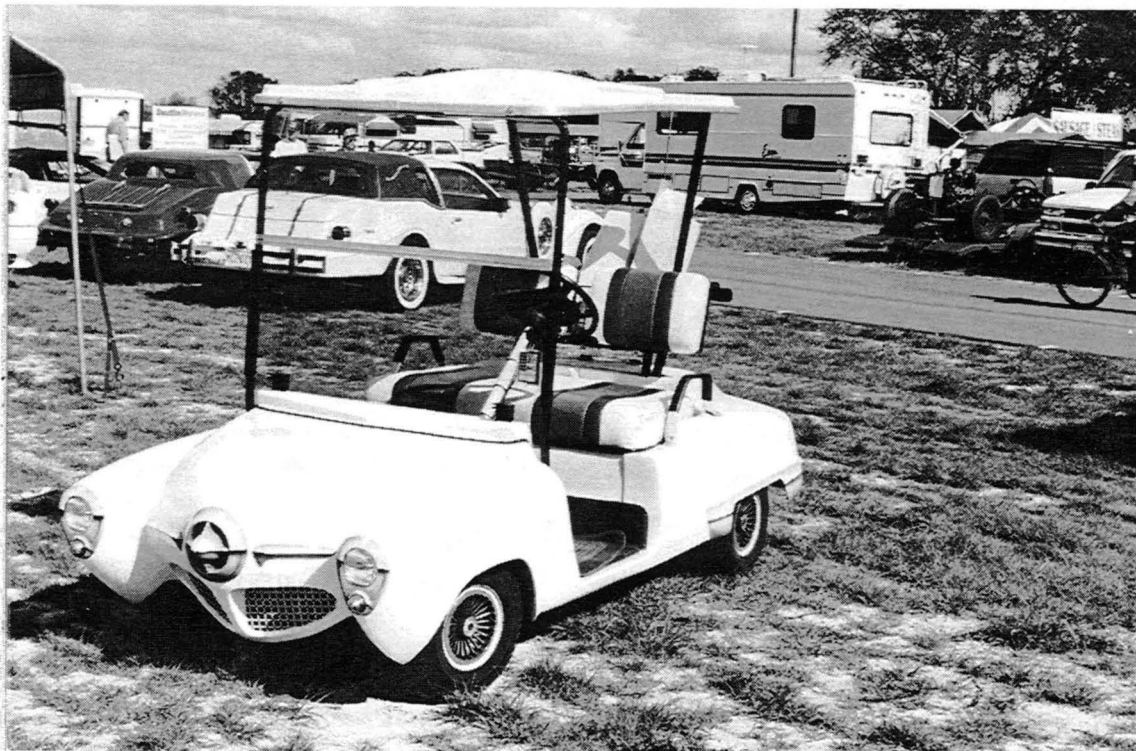
One of the most interesting ways to haul your golf clubs around. This 1996 Golden Classics is based on the chassis of an E-Z-Go gasoline-powered golf cart. The fiberglass body has been formed to look like the Raymond Lowey-designed 1950 Studebaker Champion.
