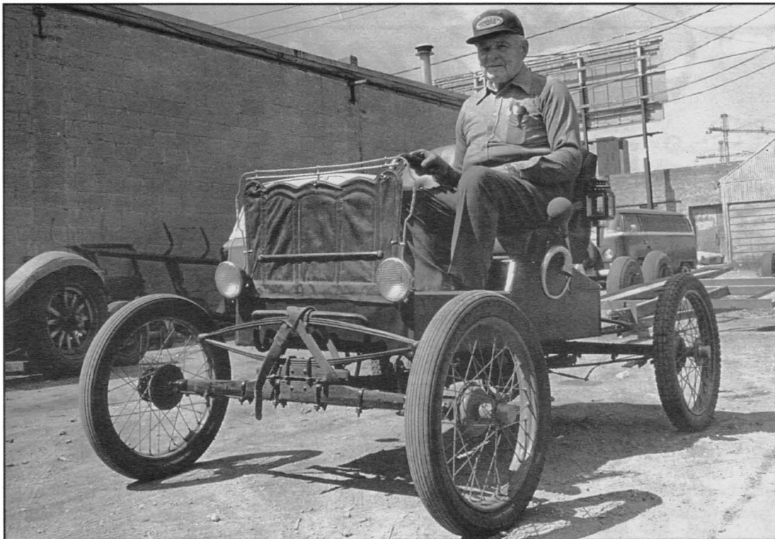
MECHANIC HENRY MILLER built his red 30-inch-wide gas-powered Millermobile, fashioned after a horse-drawn buggy, at Regina, Saskatchewan, Canada, in 1970. It has a 1911 Hamilton chassis by International, a five-horsepower Briggs and Stratton engine, motorcycle wheels, and it comes complete with headlights, taillights, kerosene park lamps, a bugle horn and Mustang insignia. It has been driven in parades, one celebrating Saskatchewan's 75th anniversary. George W. Green collection
