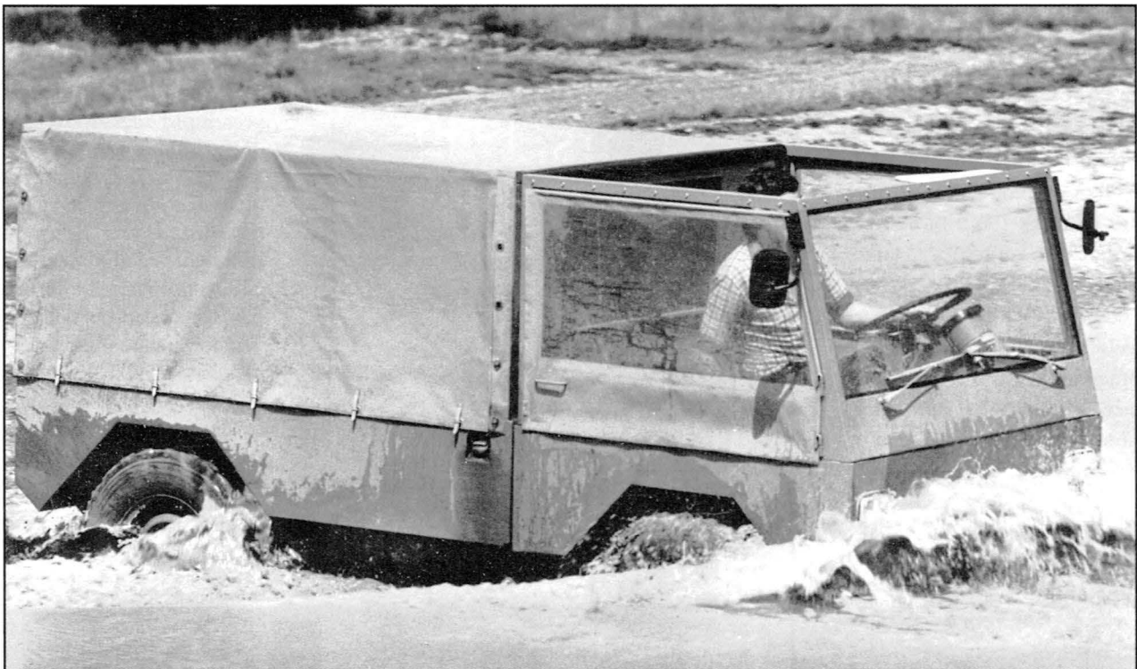
CHICO GOES FOR A SWIM —The Chico, a “cross country-mutipurpose-utility-vehicle,” was built in Buncrana, Ireland, in the 1980s by ATW Auto—Montan—Werke Ltd. Apparently a Messerschmitt design, it was powered by a rear-mounted two-cylinder Deutz diesel. The chassis was jointed behind the cab for agility on uneven terrain. Has anyone ever seen one? Kit Foster collection.
