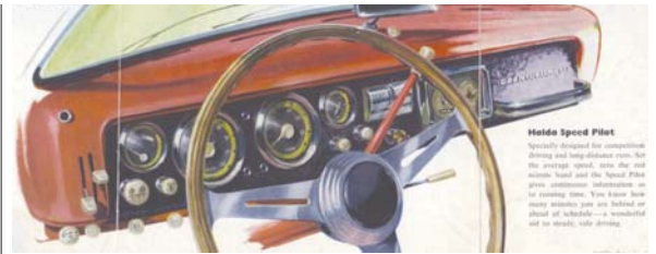
Above: SAAB offered the Halda Speed Pilot on the Granturismo 750 as a factory-installed accessory, circa 1959. To be fair, this was mounted on the passenger side, as it would be used by a co-driver.
