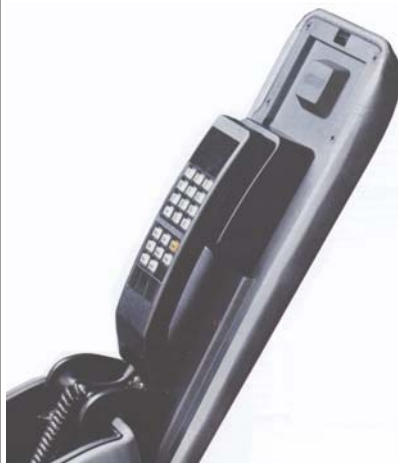
Above: With the 1986 generation IV Fleetwood, Cadillac offered a factory-installed cellular telephone with a handset concealed in the front seat center armrest. A hands-free microphone was part of the system along with an "exclusive radio mute module."
