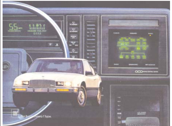
Above: The 1986 Buick Riviera featured a touch-screen display to control the radio and climate control system, seen at top right. This display was a cathode ray tube which presents some handling difficulties during repairs.
