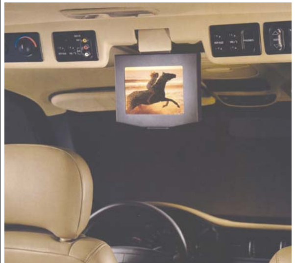
Below: For rear passengers, Oldsmobile offered a VHS video player with a fold-down color liquid crystal display in the 1999-model Silhouette Premier.
