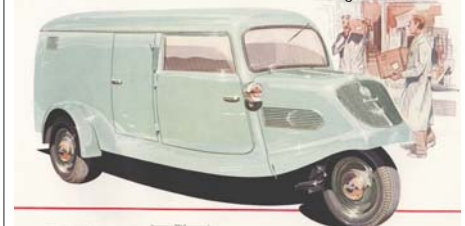
Tempo Hanseat van (above). Load area 54 x 88 inches, 44 high, 14 feet long total, the smallest version. 2-cylinder 2-cycle 396cc engine, water cooled, mounted above and steering with the front wheel, enclosed chain drive.
