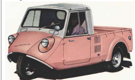
Mazda TEA 43 (above). Air-cooled 577cc V-twin engine, mounted behind the cab. Brakes only on the rear wheels. Load area 44 x 46 inches. Claimed payload 661 pounds. Smaller 356cc engine was standard.
