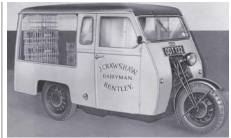
Reliant 10cwt van (above). 747.5cc inline four, side valve, water-cooled. Load capacity 20 crates of milk bottles weighing 54 pounds each. Brakes on all wheels.
