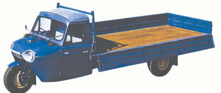
Mazda TUA 32 S (above). One of the largest postwar three-wheelers. 4-cylinder, 4-cycle 1484cc water-cooled engine mounted under the cab. Load area 160 x 61.6 inches, claimed payload 4409 pounds, with 24.7 MPG.
