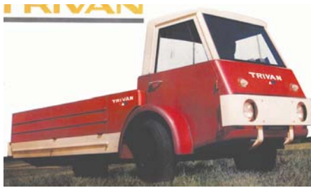
The early-1960s Trivan by Roustabout (above). The vehicle had an opposed-twin air-cooled engine. Cargo bed was 96 x 60 inches, a claimed 50 cubic feet.
