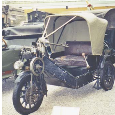
Bond Ranger (above). 250cc two-cycle powerplant cantilevered ahead of the front wheel. Steering pivots 90 degrees each direction; the vehicle turns in its own length. Wheelbase 66 inches on 132-inch total length.
