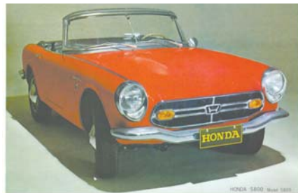
Above: 1968 Honda S800, 791cc, DOHC, water-cooled engine, 70 hp at 8000 rpm. Live rear axle. Federalized, but limited imports. Below: 1970 Honda N600, 598.7cc, air-cooled, OHC twin, front drive, 80 mph, 42 mpg. Odd three-dimensional gear selector pattern, plastic trunk lid.
