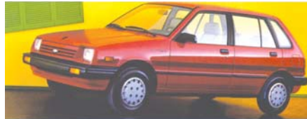
Above: 1985 Chevrolet Sprint, also Suzuki Forsa and Pontiac Firefly. SOHC, 3 cylinder, 993cc, all-alloy engine, front drive, coil strut and leaf spring suspension.
