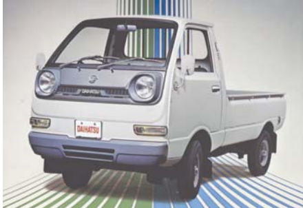
Below: 1971 Daihatsu 360 Cab, 356cc, 2 cylinder, 2 stroke engine, 350kg (772lb) payload. For non-street use.
