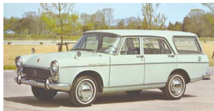
Above: Isuzu Bellel station wagon, circa 1962. Diesel, OHV, 2 liter, 4 cylinder engine, 55 hp, 89 ft-lb torque to move a 3144 lb vehicle. Isuzu's first independent design. Offered by Roger Sagner's Motor Mart, Portland, OR.
