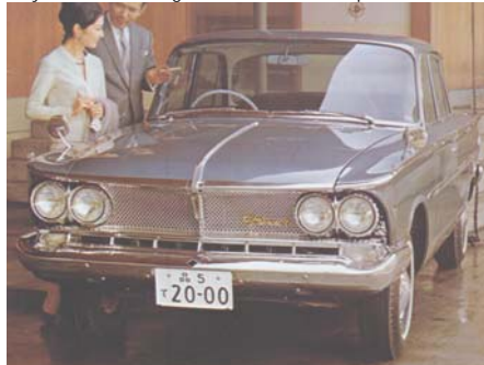
Below: circa 1964 Prince Gloria Super 6, S41D-1. SOHC 6 cylinder, 2 liter engine, DeDion rear suspension.
