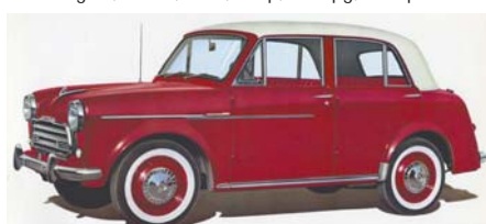
Below: circa 1964 Prince Gloria Super 6, S41D-1. SOHC 6 cylinder, 2 liter engine, DeDion rear suspension.
