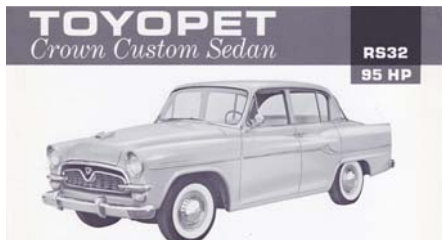
Above: Toyota Motor Distributors offered the 1.8 liter, 4 cylinder Crown starting 1958. Equipment included tinted rear view mirror, 2-speed wipers and fresh air heater.
