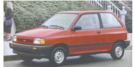
Above: 1988 Ford Festiva. Developed with Mazda, built by Kia, SOHC, 1.3 liter, 4 cylinder engine, front drive.
