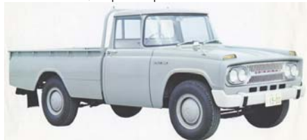
Above: Toyota Stout circa 1968. Bed size of 87.7 inch length, 62 inch width. Gasoline 4 cylinder, 1.8 liter engine. Below: Land Cruiser has had solid sales since 1961.
