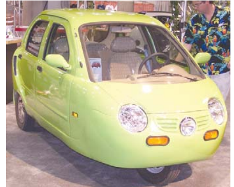
Below: Xebra electric car as seen at the Los Angeles Auto Show, January, 2006. Manufactured in the People's Republic of China. Four door, four passenger three-wheeler. Compact dimensions, 3.12m (123") length, 1.6m (63") width and height, empty weight 1441 lbs. Onboard charger, motor above the rear axle, 25 mile range, 40 mph top speed. Uneven fiberglass, crude engineering and execution of interior finish. Several facelifts and addition of a rear hatch evident by 2010. Often seen as delivery vehicles with large appliqué graphics on the sides.
