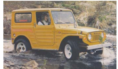
Below: 1972 Suzuki Brute IV, L50 water-cooled, 2 cylinder, 2 stroke, 356cc engine. Rugged all-steel styling belied by hilarious ring-a-ding exhaust note. Several air- and water-cooled engines offered, with two or three cylinders.
