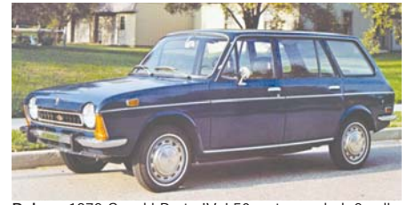
Below: 1972 Suzuki Brute IV, L50 water-cooled, 2 cylinder, 2 stroke, 356cc engine. Rugged all-steel styling belied by hilarious ring-a-ding exhaust note. Several air- and water-cooled engines offered, with two or three cylinders.
