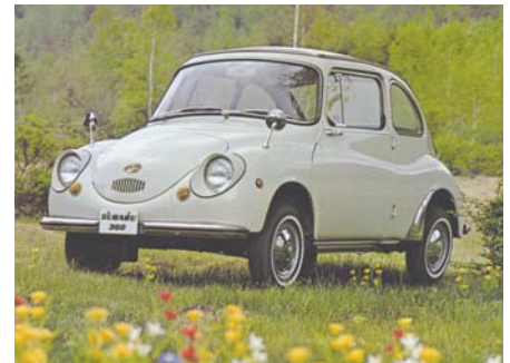
Above: Subaru 360, produced 1958-1971, air-cooled 356cc, 2 cylinder, 2 stroke, rear engine. Torsion bar and coil spring independent suspension. Exempt from federal safety standards by 925 lb weight. Below: Subaru Star, imported beginning 1970, horizontally opposed, water cooled, 1088cc engine, front wheel drive with inboard brakes. Independent torsion bar and coil spring suspension. Imported by Bricklin and Lamm's Subaru of America.
