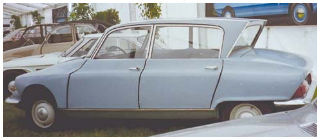
Citroën C 60 prototype, below, and right. The production Ami 6 used coil spring suspension similar to the 2CV while the C 60 proposed hydropneumatic suspension.
