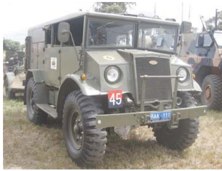
The Canadian Military Pattern trucks, number 13 cab design, above. These versatile vehicles featured a reverse-angle windshield to minimize sun reflections in the flat glass which would be observable by air. Primarily built by Ford and Chevrolet, the vehicles were made in dozens of configurations, and like all military vehicles, could be built in several nations simultaneously. This Ford CMP Blitz truck is shown at the Barossa Air Show in South Australia, photo by GTHO.
