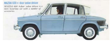
Mazda Carol 360 and 600 series, above and top. Circa 1962-1970. Restricted to 118 inches length by law, creating a four-door sedan would be challenging without a reverse-angle rear profile. The Carol 360's 358cc 4-cylinder OHV rear engine was one of the smallest production fours.
