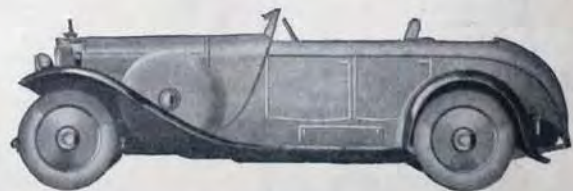
Model S, two passenger torpedo, transformable "Bretche" illustrated above, is capable of speeds up to 120 miles per hour. Model K, 4 passenger torpedo, transformable sport, at the right will attain 110 miles per hour. Upholstered in Alpina genuine Lizard. Coachwork of both models by J. Saoutchik of Paris.
