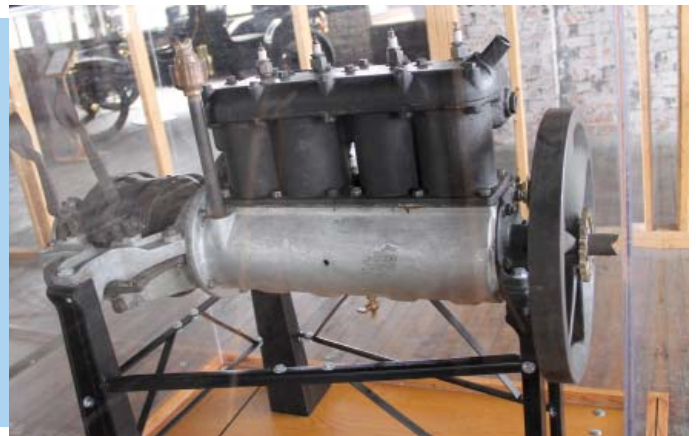
Left: a 1906 Ford Model N Prototype Engine. Right: a 1908 prototype engine based on the N engine but with a removable cylinder head, paving the way to the Model T. Note the 2x4s in both photos marking out the footprint of the 3rd floor experimental room at Piquette.
