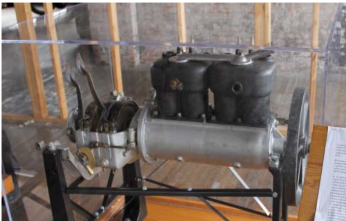
Left: a 1906 Ford Model N Prototype Engine. Right: a 1908 prototype engine based on the N engine but with a removable cylinder head, paving the way to the Model T. Note the 2x4s in both photos marking out the footprint of the 3rd floor experimental room at Piquette.
