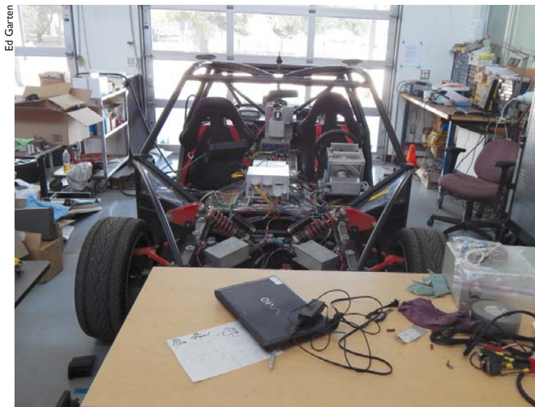
This is the X1 Experimental Vehicle, a project of Stanford's Dynamic Design Lab. The goal is to develop a second-generation drive-by-wire vehicle, building on previous steer-by-wire experiments.
