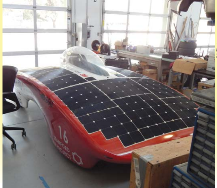
This is Luminos, a creation of the Stanford Solar Car Project. It cruises at 45 mph in full sunlight, and its batteries allow it to go 150 to 200 miles in diminished sunlight. For details, see: solarcar.stanford.edu .
