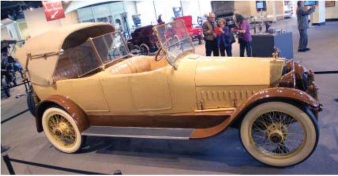
Before the Chevy Volt, there was the Owen Magnetic. This 1916 example uses a petrol engine to power an electric motor.
