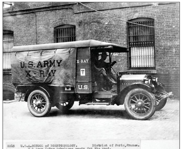
GMC built over 5000 ambulances on its Model 15 and Model 16 chassis. The one shown here was used for X-ray services, a new medical procedure in WWI.
