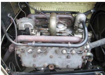
The 314.5 cid 70 hp side-valve (L-head) Cadillac V8 was introduced in 1915 and was used in all Cadillac staff cars. The horsepower was raised to 77 hp in 1916.
