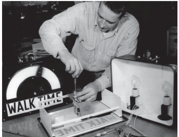
Douglas B Hutchings assembling the Walk Time prototype. Note the earliest type incandescent light bulbs.
