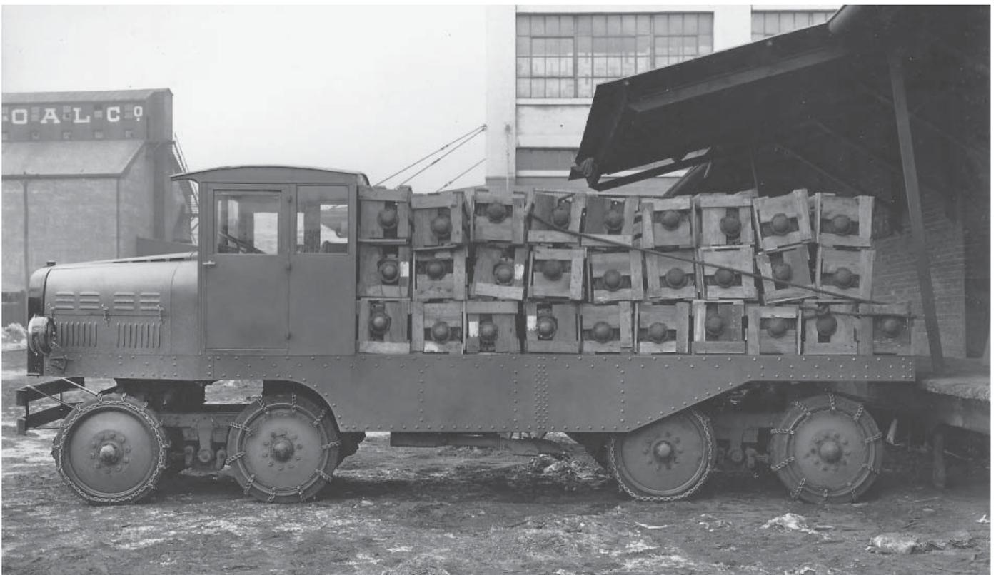
As seen in *SAH Journal* No. 307, this is believed to be a Versare bus chassis used at the factory for carrying parts, in this case axles.
