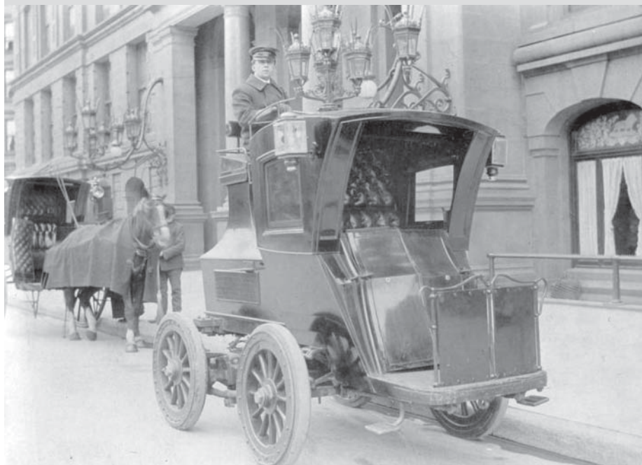
This photo of an Electric Vehicle Company hansom cab was taken in 1904. Of particular note is the similarity with the horse-drawn hansom cab just behind it, upon which the electric version was based. For more on these electric cabs see SAH Journal #302, pp. 8-13.
