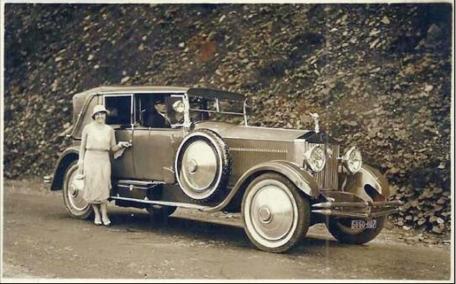
A Rolls-Royce Silver Ghost rebodied by Franay circa 1929, fitted with Cromos flèche d'argent bumpers.
