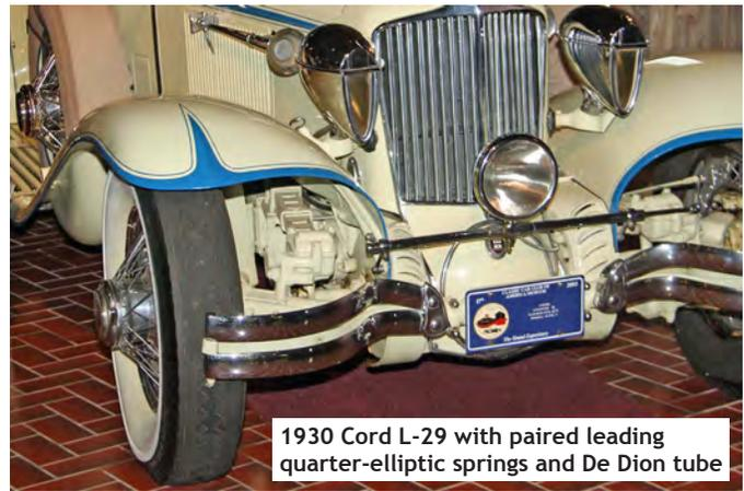
1930 Cord L-29 with paired leading quarter-elliptic springs and De Dion tube
