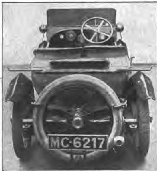
Rearward view of the 12 h.p. 1920 Bugatti, showing the attachment of the reversed quarter-elliptic springs to the tubular rear cross-member
