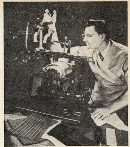
*This testing machine finds out how well automobile seat cushion upholstery will wear against the material from which suits and overcoats are made. Strips of the upholstery are rubbed against the suit material until the wearing qualities have been determined.*
