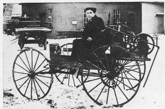
Bill Gray, age 14, and the car he built in 1905. It was powered by a steam engine converted to gasoline.
