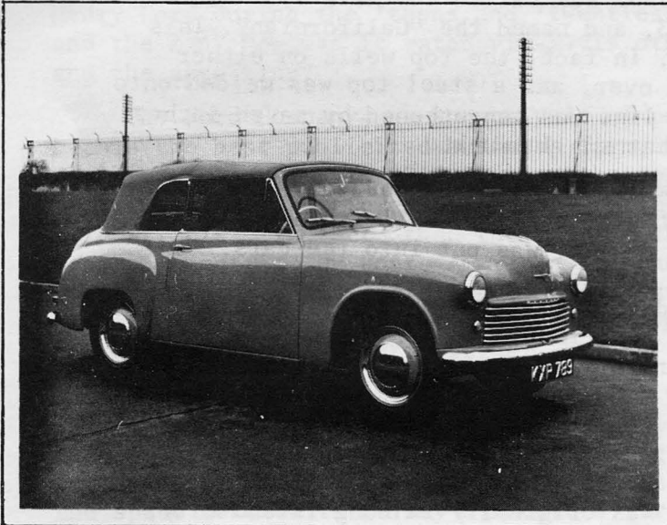
1951 Mark IV Convertible. Note "Trafficators" behind door.
