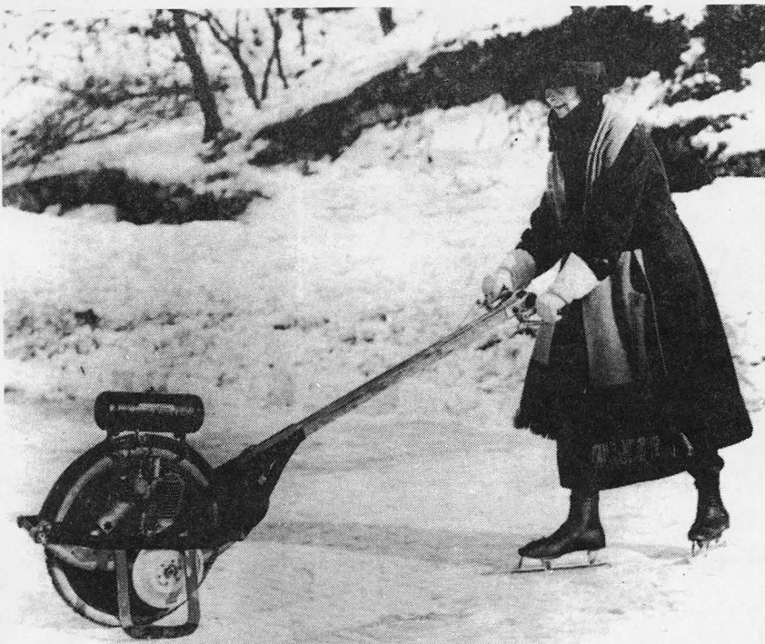
Ice Skater Towing Device using a Briggs & Stratton Motor Wheel, no year given.
