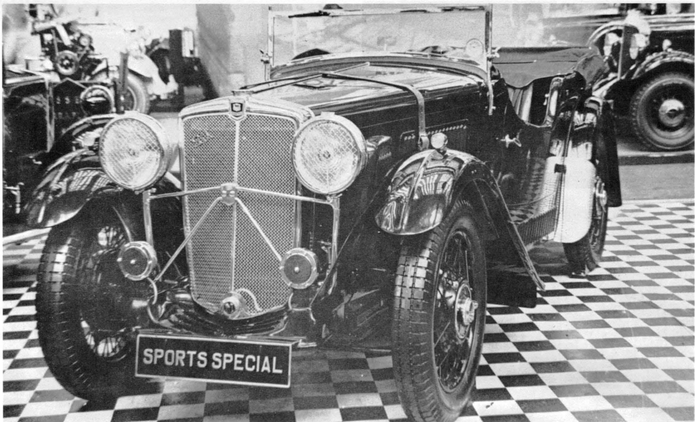
Factory Photograph: The "Sports Special" is a 1934-35 Morris 1016, that featured an L head 6 cylinder engine with twin carburetors. Photograph from the collection of the editor.
